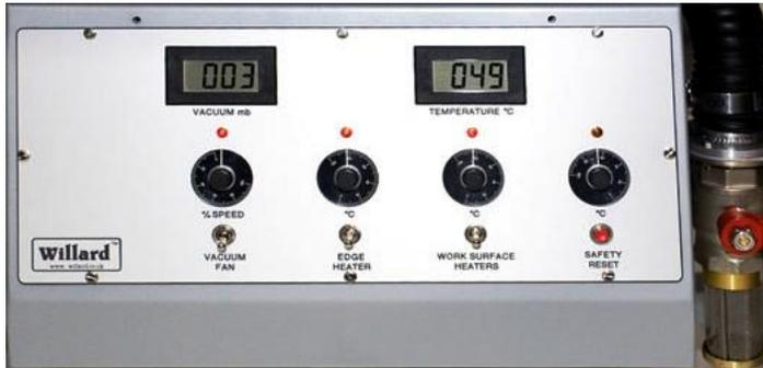
*Top Row: Pressure differential readout, work surface temperature readout*
